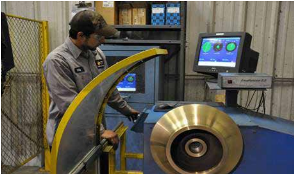
All Impellers & rotating elements dynamically balanced
