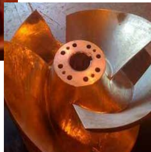
Finished Machined and Balanced Impeller
